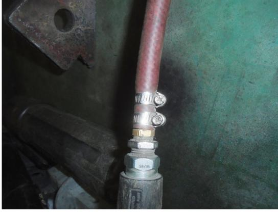
Absolutely not! The air hose pictured is secured with a worm gear hose clamp, which is not suitable for this use. Such clamps can fail, potentially exposing employees to dangerous whipping actions from the hose. This is a recognized hazard, with OSHA often citing violations under standard 1910.243(b)(2).
