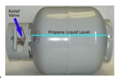
allows pressure to be safely vented (i.e. temperature increases). In the picture above, the liquid level is above the pressure relief valve. This would not allow the cylinder to vent properly.
