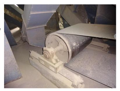
Hazards associated with nip and shear points must be guarded. Side guards can be installed to prevent employee contact with power transmission components, in-going nip points, and the conveying medium. Secondary safeguarding methods may include the use of standard railings or barrier fencing, pre-start up signals, and warning signs.
